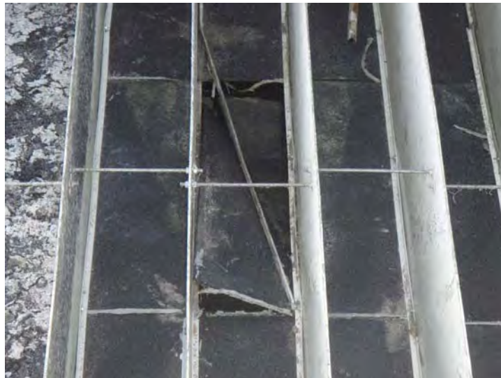
Figure 2.1: Sundog Filter Porous Plate Failure
