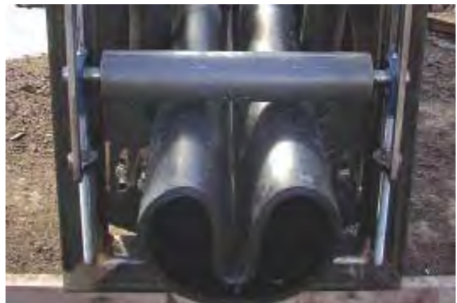
Figure 3.1 PE Pipe in Insituform Polyfold Machine
