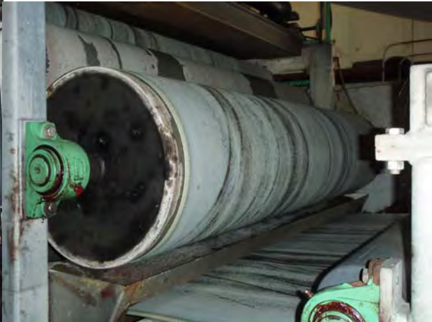
Figure 3.4 Struvite on BFP Belt and Rollers
